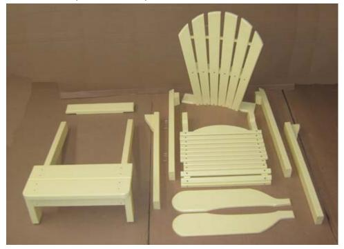
Remove the screws from the bags. A square drive bit is included. Start the screws into the countersunk holes on the pieces. The two shorter screws are for the bottom of the back section. Advance the screws into the holes until they protrude <u>slightly</u> from the other side. The protruding screws will help you line up pieces when assembling.
