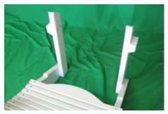
Step 2:: For the remaining pieces advance the screws until they protrude the other side slightly - this will help line up the pieces easier to their original holes. Attach rear legs - notice which way the top of the legs point.
