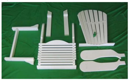
Remove the screws from the bag. Start the screws into the countersunk holes on all the pieces. Note: the 4 shorter screws are for the bottom of the back section. The longer screws go in all the other countersunk holes. There are 2 extra long screws included in case you need them. Advance the screws into the pieces but do not let them protrude the other side at this time.
